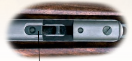
The fore-end incorporates an interchangeable insert in special hardened steel that makes it easy to tighten the shotgun if it becomes loose through years of very heavy use
