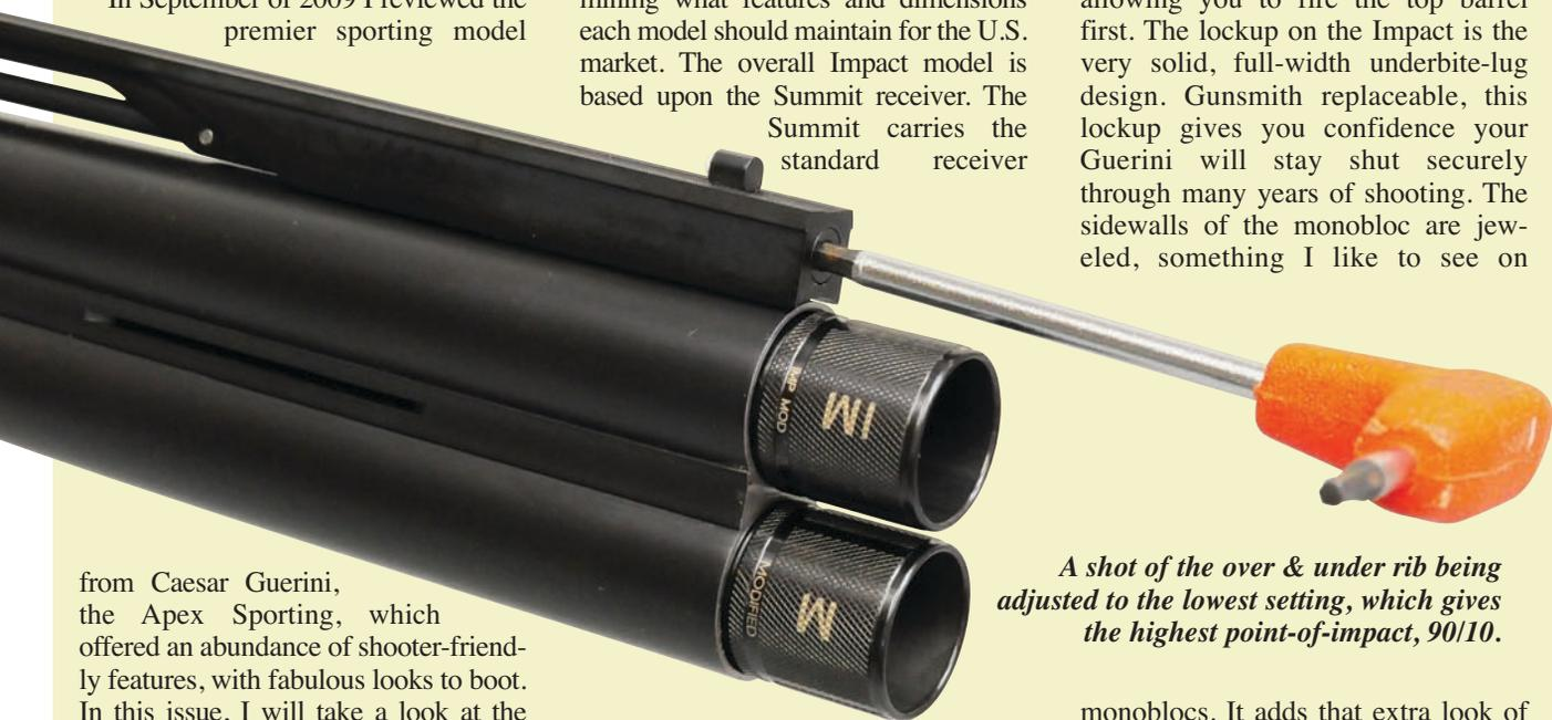
*A shot of the over & under rib being adjusted to the lowest setting, which gives the highest point-of-impact, 90/10.*
