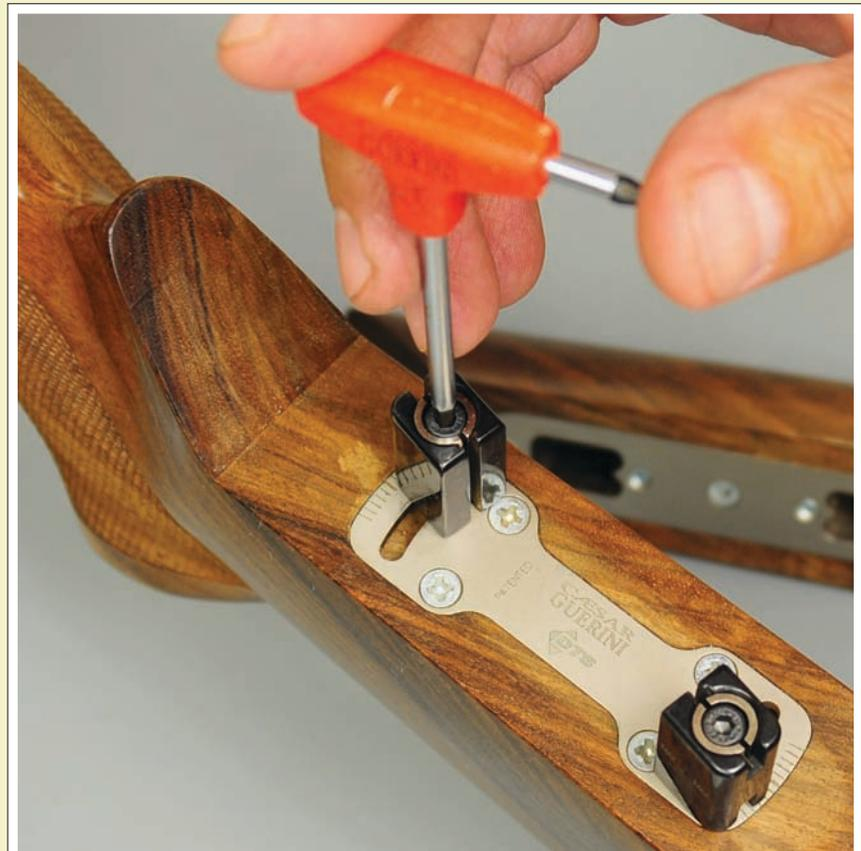
*A view of the Impact's adjustable-comb hardware. Lateral movement of the comb is ⅝" and maximum vertical range is .55". This is another component of the Guerini Dynamic Tuning System (DTS).*
