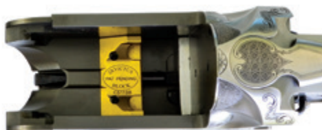
The innovative, replaceable and patented Invictus Block attaches to the receiver floor and engages the monoblock lugs to hold the barrels back against the breech face.
